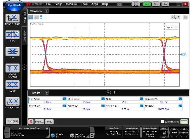
Data Rate = 2.5 Gb/s,  $V_{in} = 220 \text{ mV}_{pp}$
