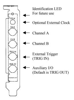
You can use CH A and CH B to digitize data as well as to trigger an acquisition.
