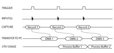
NOTE 1: No Trigger Events Are Missed - Guaranteed NOTE 2: Over 95% of CPU cycles are available for data processing
