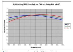
We measure every transmissive VPH grating to ensure exceptional 1st order diffraction efficiency uniformity over the specified operating band. Not all vendors do!
