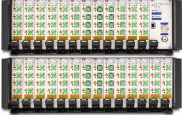
This series of mainframes host our *CoBrite<sub>MX</sub>* tunable laser modules. All variants can be equipped with handles and rubber feet for bench-top use or brackets for 19inch rack mount usage.
